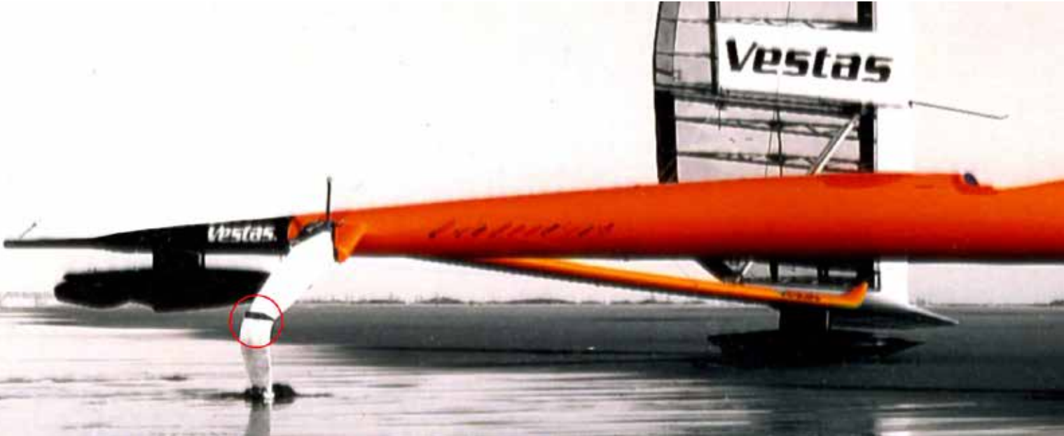
The fence can be seen on the top of the foil just above the bend in the foil. Photo: Helena Darvelid
